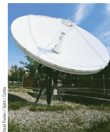
(a) A satellite dish reflects signals to the focus of a paraboloid.
